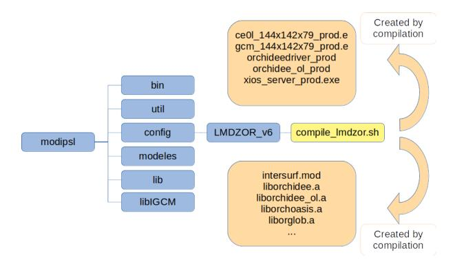
In the case of LMDZOR\_v6 configuration, the executables <u>orchideedriver\_prod</u> and <u>xios\_server\_prod.exe</u> are specific to the offline model. In the following exercises we will use the coupled configuration and ce0l, gcm, and xios server executables.
